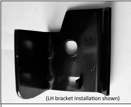
This support bracket is designed to minimize mirror vibration as the door was not originally designed for this towing mirror.
